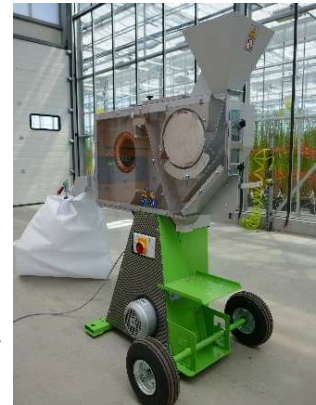
Adaptable laboratory grain thresher
